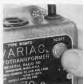
Overload protector, a feature on portable models, is reset from front panel.
